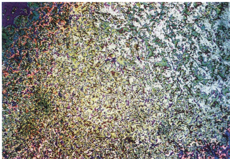
Figure 9. Photomicrograph of: \text{NC}-\text{C}_6\text{H}_4-\text{C}\equiv\text{C}-\text{C}\equiv\text{C}-\text{C}_6\text{H}_4-\text{N}=\text{CH}-\text{C}_6\text{H}_4-\text{OC}_2\text{H}_5 showing the appearance of a nematic texture at c. 200°C.
